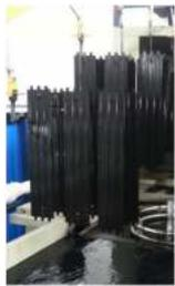
The evaporator and condensing coil are coated with corrosion protection (Hot Dip)
